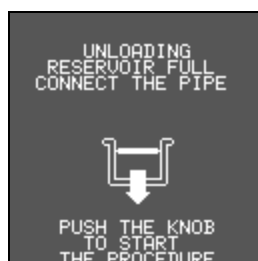
fig. 21 – "DISCHARGE TANK FULL" warning screen
