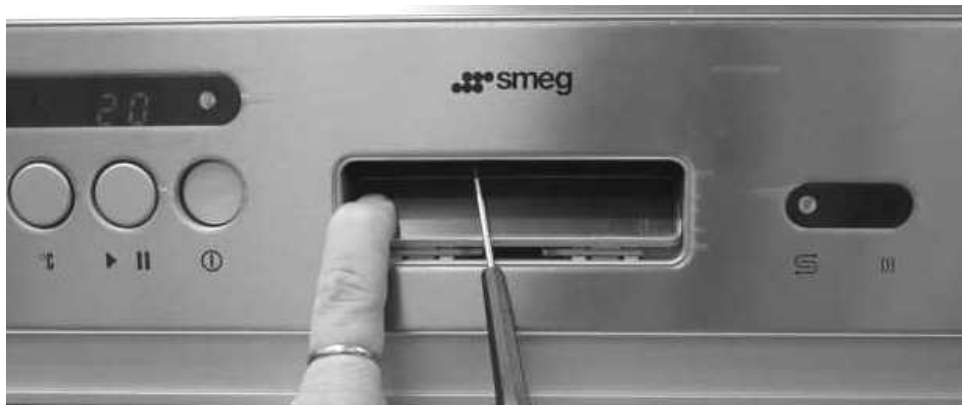
fig. 2 – WD1050 front. To unlock the door manually: 1 - push the handle opening to access the opening mechanism, 2 - Force, pushing it from bottom to top, with a small screwdriver the opening mechanism.
