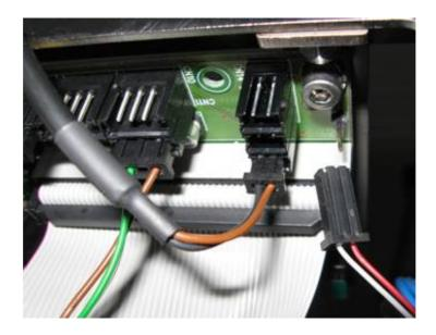
Connect the calibration tool 2-pin cable to the connector CN12, CN13 or CN14 of the *power cable 34.* Switch pole number 1 of the temperature selector to ON, which corresponds to a 1000 Ohm sample coil (0°C).
