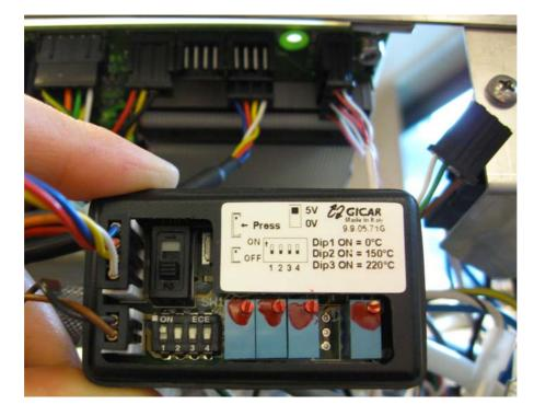
Connect the calibration tool 4-pin cable to the connector CN11 of the *power cable 34*. Set the calibration tool switch to 0 V (position 2).
