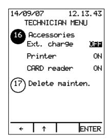
Select Accessories (option 16) and press ENTER. The external charge value (ON/OFF) will appear. Press  $\uparrow\downarrow$  to change the value, press ENTER to confirm and move to the next option.
